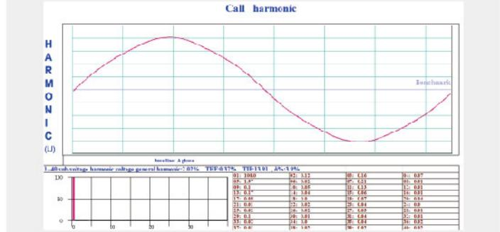
This generator tester can measure most electric parameters of a single-phase or three-phase AC generator. The standards it complied with are GB/T 2820-1997 and GB 2820-90. The signal frequency can be measured varies from 45 Hz to 65Hz. You can select one wiring mode from four modes – 1Φ2W, 3Φ3W, 3Φ4W and 3V3A. The following table shows the parameters: It's the best way to replicate, prove and verify the real-life demands on critical power systems.
